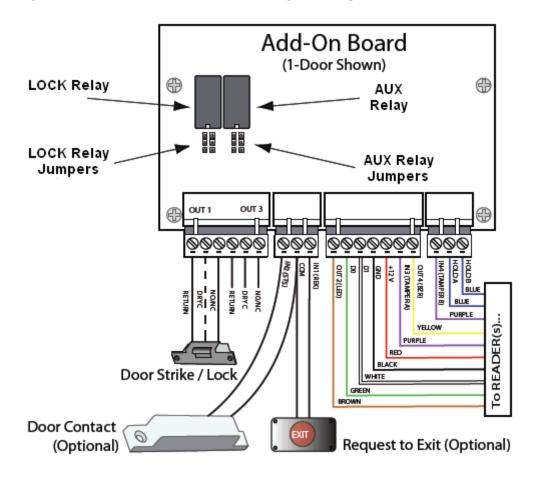
Figure 3: NetAXS-123 Add-On Board Wiring and Components
